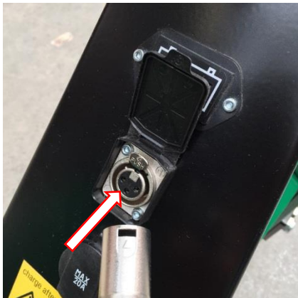
Image 6.1 – connecting battery charger
