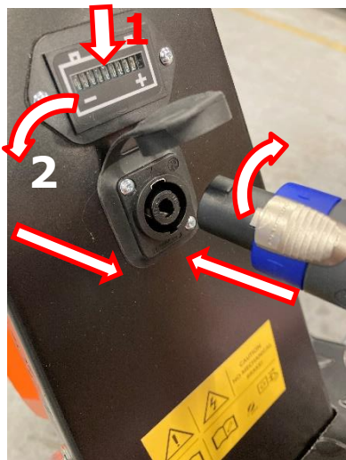
Image 6.3 – connecting battery charger
