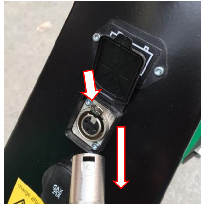
Image 6.2 – disconnecting battery charger
